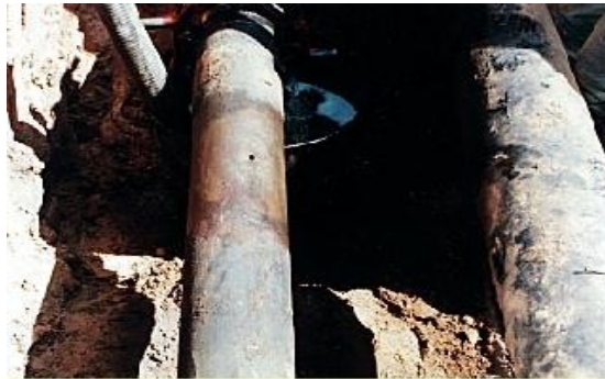
Failed pipe section shows the perforation clearly (Fig. 1).
